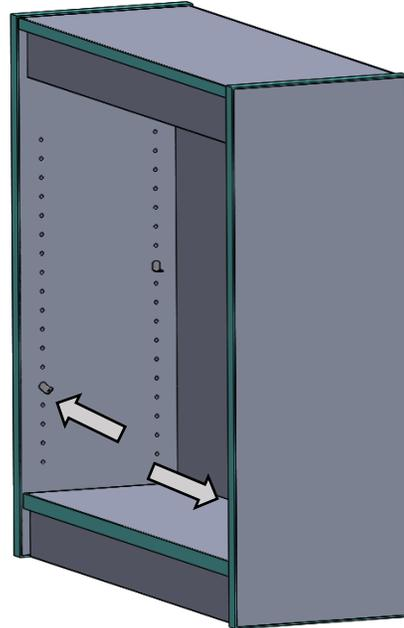
3. Set the shelf onto the rear shelf clips and attach with (2) #10 X 5/8 screws.
