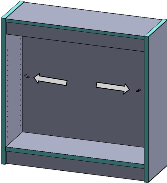
2. Insert (2) shelf clips into the front set of holes on the library end/intermediate panels, six holes lower than the rear shelf clips.
