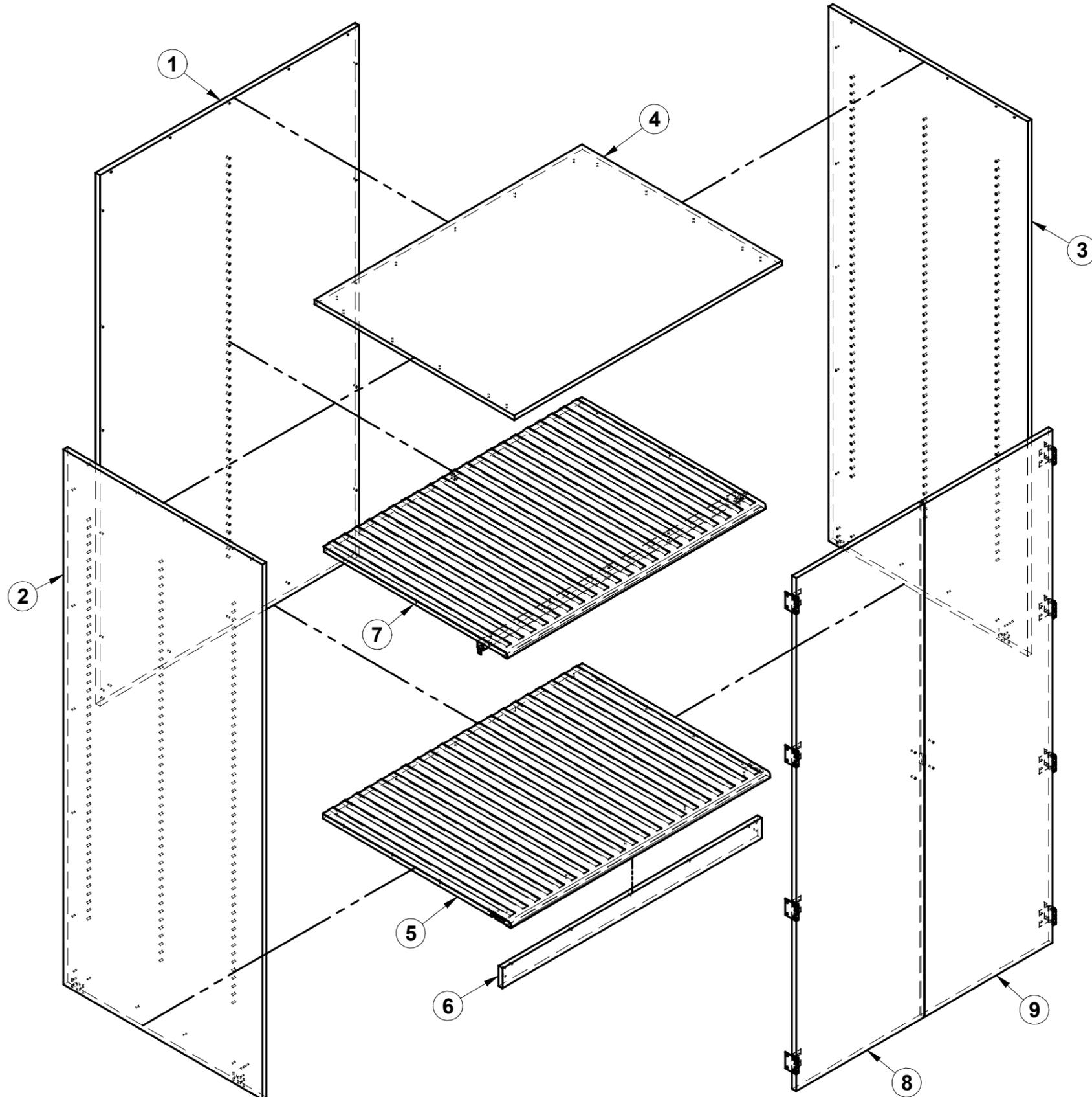
1. Attach end assemblies (2, 3) to back (1) with #10 x 5/8" pan head screws (10)
