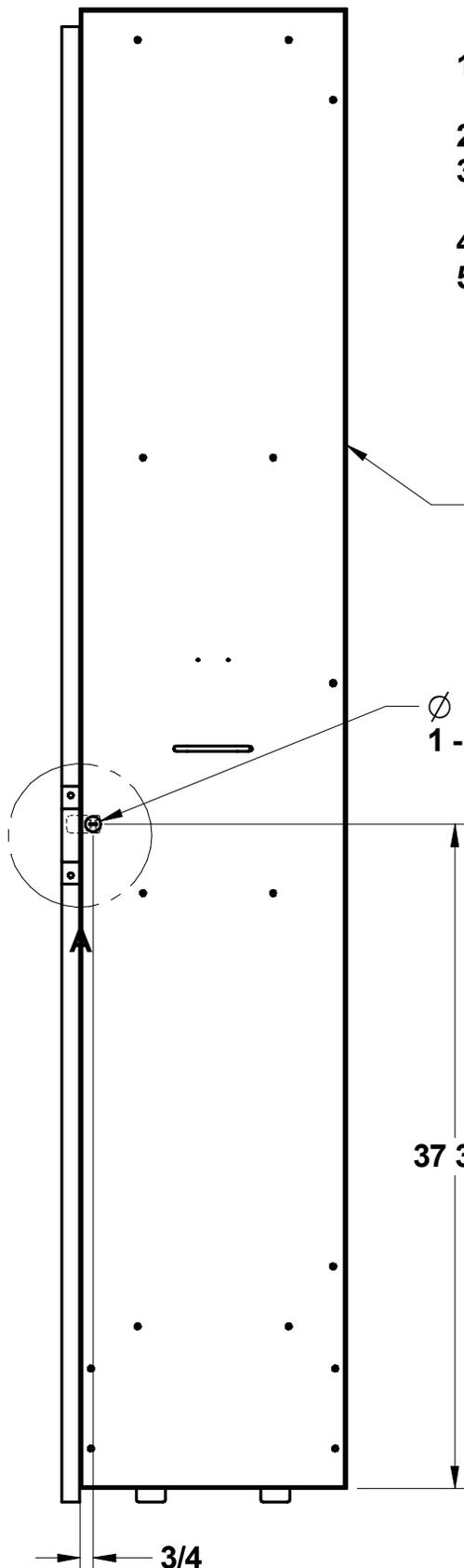
1. DRILL (1) 3/4" DIA. HOLE IN LOCATION SHOWN IN FRONT PANEL.
