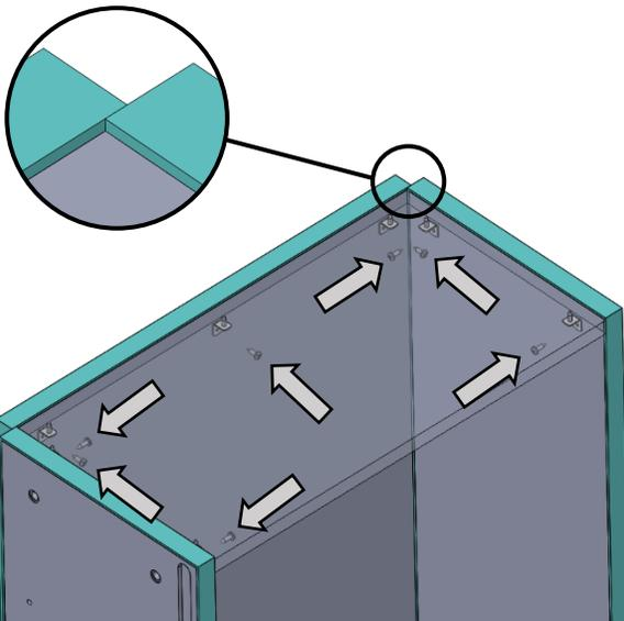
**4.** Align the second filler panel 4.25" from the bottom of the end panels with brackets facing down. Screw into the end panels using (7) #10 X 0.625" screws. Tighten to a torque of 30-35 in-lbs. Begin the library starter instructions (933710-INST) with the left hand end panel.
