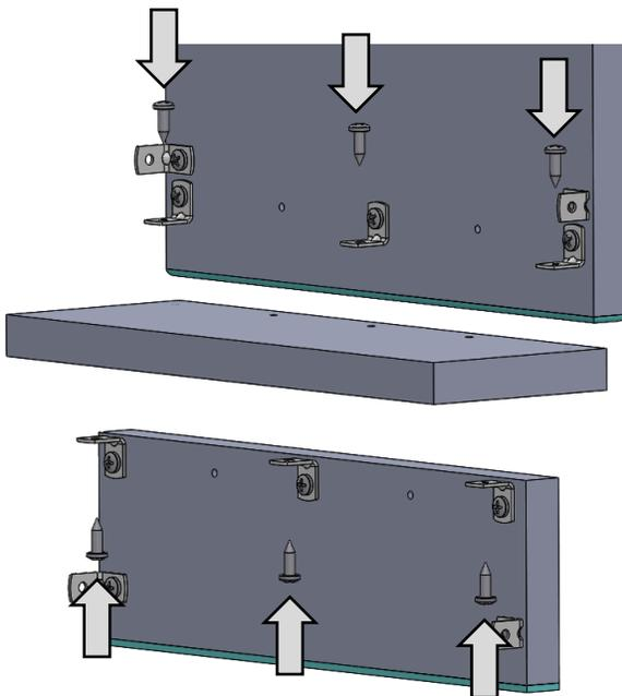
4. Attach the top panel to the front panel using (3) #10 X 0.625" screws. Tighten to a torque of 30-35 in-lbs. Attach completed filler to learning wall using remaining #10 X 0.625" screws.
