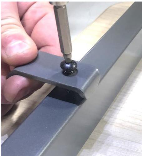
4. The bag hook is now ready for use. **The load on the bag hook should not exceed 25 lbs.**
