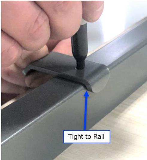
2. Drill a pilot hole in the marked location using a 1/8" diameter drill bit. This will ensure that the self-drilling screw goes in easily and in the correct location. Be sure clean up all metal shavings to prevent injury or damage to other products.
