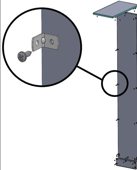
3. Attach the bottom panel to the front panel and toe kick using (6) #10 X 0.625" screws. Tighten to a torque of 30-35 in-lbs.
