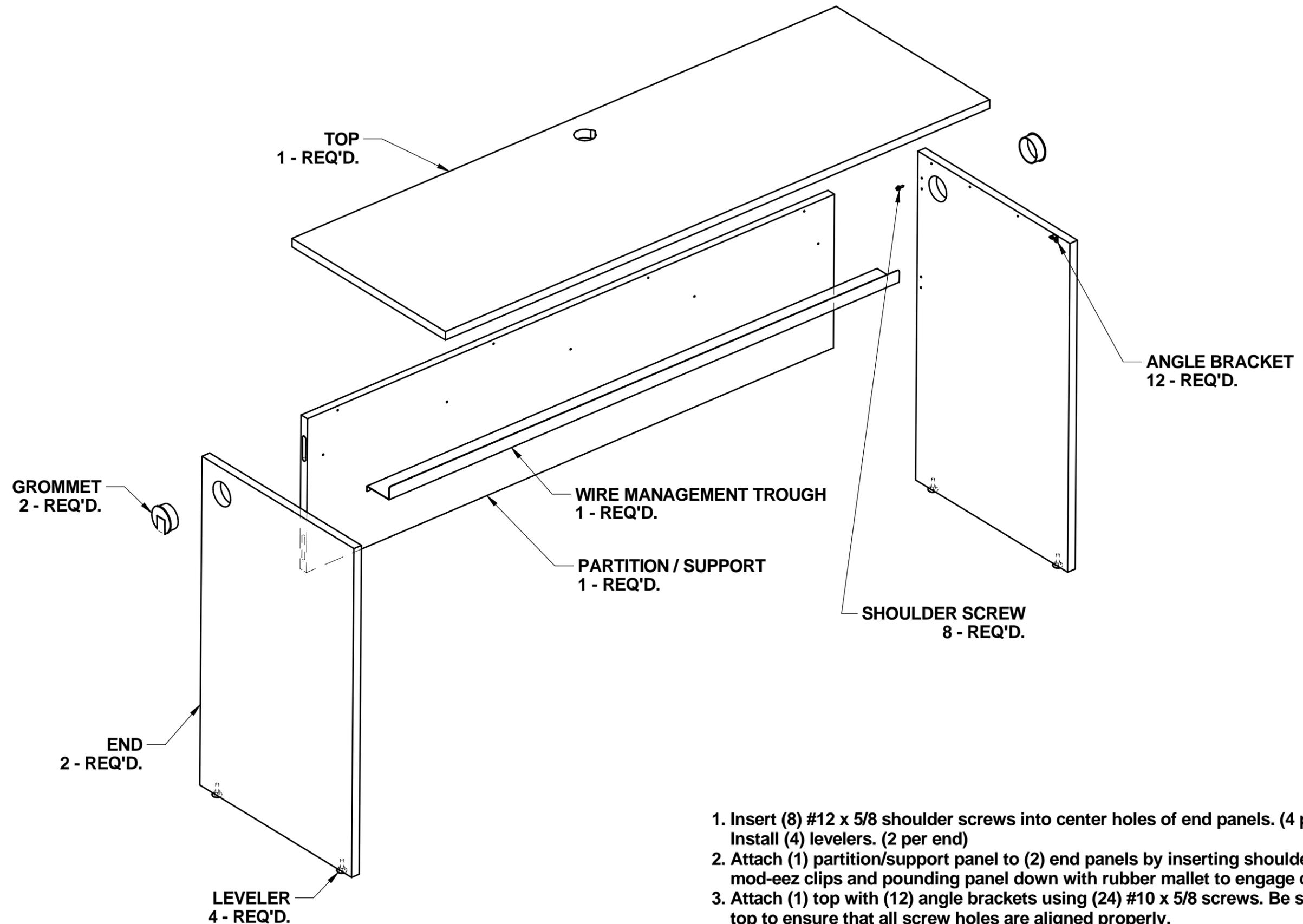
1. Insert (8) #12 x 5/8 shoulder screws into center holes of end panels. (4 per end)
