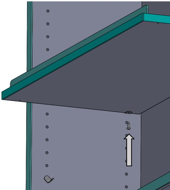
4. Tilt the shelf down until it rests on the front shelf clips and attach with (2) #10 X 5/8 screws. *Note: To change the fixed magazine shelf into a flip up shelf, do not use the front shelf screws.*
