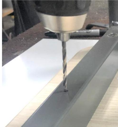
3. Attach the bag hook to the rail using the supplied self-drilling screw. Position the screw straight as you drive it in and stop once the screw head is tight to the bag hook. **Do not overtighten the screw.** Overtightening the screw will cause the threads to fail and the attachment will be unreliable.
