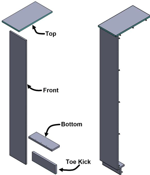
2. Attach (9) brackets to the top panel, (13) brackets to the front panel, and (5) brackets to the toe kick using (27) #10 X 0.625" screws. Tighten to a torque of 30-35 in-lbs.
