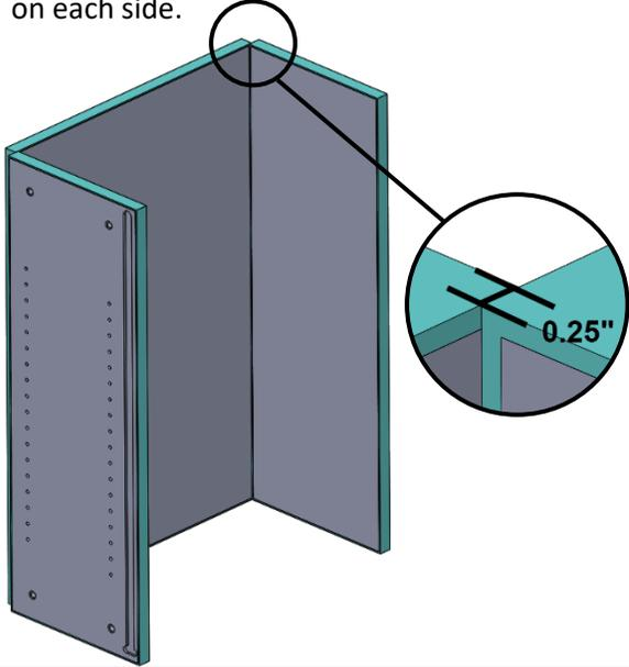
**3.** At the top of the end panels, align one filler panel with brackets facing down at the bottom of the edgeband. Screw into the panels using (7) #10 X 0.625" screws. Tighten to a torque of 30-35 in-lbs.
