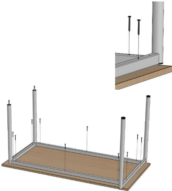
2. Attach (4) bumpers to frame using (4) #8 X 3/4" pan head screws. Tighten to a torque of 30-35 in-lbs.
