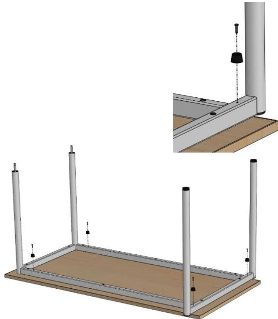
3. If table requires casters, lightly tap casters onto caster stems using a rubber mallet.
