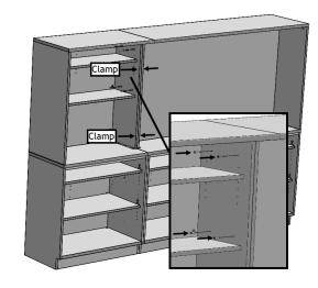
Attach the hutch to the base cabinet using (6) #10 x .750" flathead wood screws. Tighten to a torque of 30-35 in lbs.
