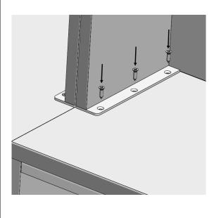
6. Use a 9/64" drill bit to predrill .5" deep holes into the base cabinet top, using the mounting plates as a guide.
